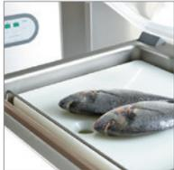
Insertion plates for volume reduction and height regulation
