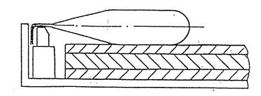
The bag opening should never be placed on the edge of the chamber as it would be pressed closed with the closing of the chamber lid. The air would then be unable to escape the bag during the vacuuming process. It goes without saying that the bag end should not be left hanging outside the chamber as this would render the vacuuming process impossible.
