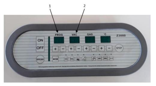
Now use the +/- pushbuttons to select programme 55 in the "PROG" display field (see Figure 1) and close the machine lid.
