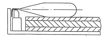
The bag opening should never be placed on the edge of the chamber as it would be pressed closed with the closing of the chamber lid. The air would then be unable to escape the bag during the vacuuming process. It goes without saying that the bag end should not be left hanging outside the chamber as this would render the vacuuming process impossible.
