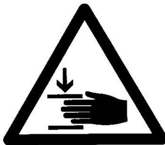
It warns that the danger zone should be clear of all persons when the machine is in operation.
